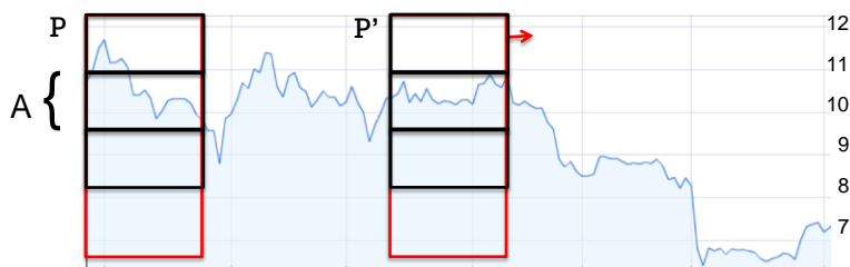
Figure 2. The A-Distance compares the probability, P , that an element in a stream will fall into the "box" with height A with the probability P' it will fall into the corresponding box at a later point in time. When the probabilities differ by more than some threshold, the system infers that the underlying distribution of the stream has changed.
