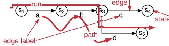
Figure 4. Examples of a state, edge, edge label, run, and path.
