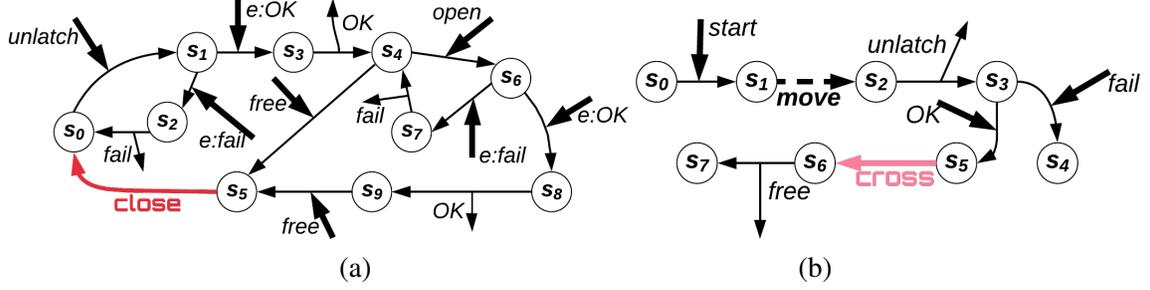
Figure 1. (a): An IOA  $\sigma_d$  for a spring door. The bold incoming arrows represent inputs of  $\sigma_d$  coming from other IOAs or the environment. The outgoing arrows represent messages sent by  $\sigma_d$  to other IOAs. The red transition ‘close’ is a command. (b): An IOA for a robot going through a doorway.
