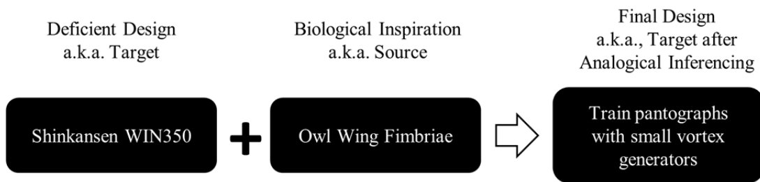
Figure 2. The analogy to owl wing fimbriae aided the redesign of the train pantographs.
